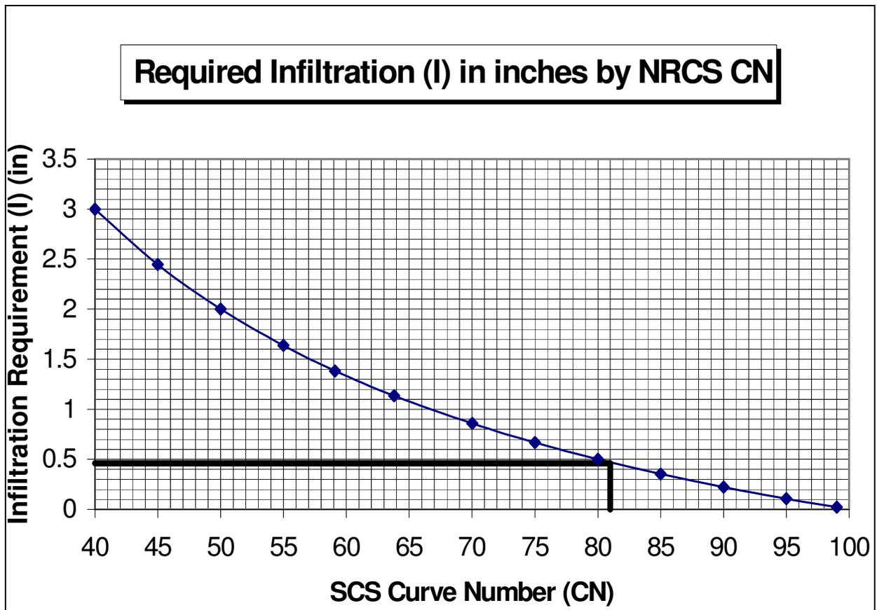
Figure 305.1. Infiltration requirement based upon NRCS Curve Number.
